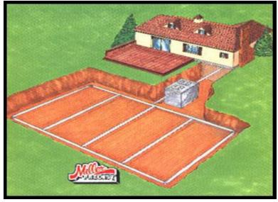
• In-Ground Trench - This system is used on properties that have a maximum slope of 25%. A standard trench absorption area consists of two or more excavated linear trenches in which perforated pipes or laterals distribute effluent into a layer of crushed stone under the pipes.
