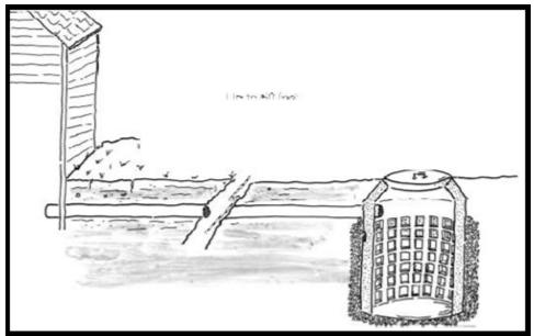
Holding Tank - A watertight tank used for sewage collection and storage. No treatment is
