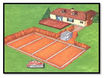
**In- Ground Trench-** This system is used on properties that have a maximum slope of 25%. A standard trench absorption area consists of two or more excavated linear trenches in which perforated pipes or laterals distribute effluent
